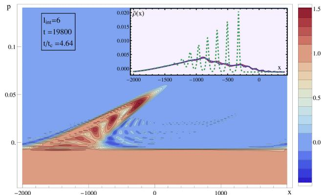
FIG. 2: Quasiparticle phase-space distribution (Wigner function) for a short interaction range,  $l_{\text{int}} = 6/mv_F$ , at  $t = 4.6t_c$ . Inset: corresponding density (solid red line) in comparison to the density of non-interacting fermions (green dotted) and the predictions of classical hydrodynamic theory (dashed blue).
