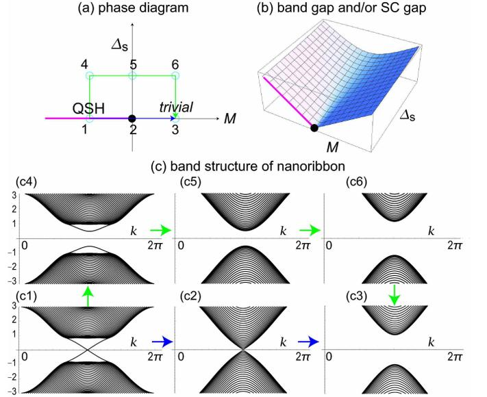
FIG. 7: (a) Topological phase diagram in the  $(M, \Delta_s)$  plane. The horizontal axis is the Dirac mass  $M$  and the vertical axis is the superconducting gap  $\Delta_s$ . The vertical axis is the energy in unit of  $B$ . We have set  $A = B = 1, C = D = 0$ . See also the caption of Fig.2.
