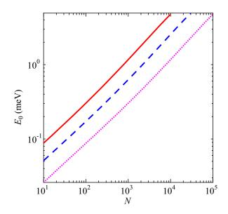
FIG. 10: The ground state energy  $E_0$  vs the number of IXs *N* for the 1D problem. Three lines (magenta dotted, blue dashed, and red solid) correspond to the 1D interaction parameters  $g_{1D}(N)$  shown in Fig. 9 by the same colors and, in turn, to 2D interaction parameters g = 2 (magenta dotted), 7.1 (blue dashed), and 20 (red solid)  $\mu$ eV ·  $\mu$ m<sup>2</sup>.
