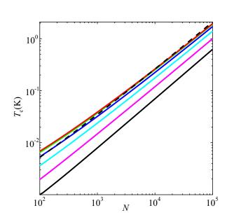
FIG. 8: Numerical simulations for condensation temperature  $T_c$  vs the number of IXs N for IXs in the rectangular trap with infinite walls for different side ratios  $a_1/a_2 = 1, 2, 4, 8, 16$ , and 32 (red, green, blue, cyan, magenta, and black solid lines, respectively) and the same area  $A = a_1a_2 = 105 \ \mu\text{m}^2$ . Black dashed line marks analytical estimate  $T_{c-\text{rectangular}} = T_d / \ln N = \frac{2\pi \hbar^2 N}{mA \ln N}$ .
