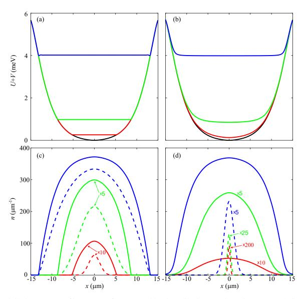
FIG. 6: (a-b) The IX energy profile in a 1D trap for T = 50 mK (a) and 10 K (b). The IX number in the trap N = 75 (red), 750 (green) and 7500 (blue). The bare trap energy profile is shown by black line. (c,d) The corresponding IX density distributions n (solid) and ground state density distributions  $n_0$  (dashed). For the screened trap in (a-d), the 1D interaction parameters correspond to the 2D interaction parameter  $g = 20 \ \mu \text{eV} \cdot \mu \text{m}^2$  as described in the text.
