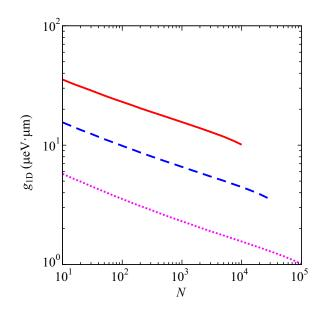
FIG. 9: One-dimensional interaction parameter  $g_{1D}$  vs the number of IXs *N* for three two-dimensional interaction parameters g = 2 (magenta dotted), 7.1 (blue dashed), and 20 (red solid)  $\mu$ eV ·  $\mu$ m<sup>2</sup>. For fixed *N* and *g*, the 1D interaction parameter  $g_{1D}$  is such that chemical potentials  $\mu$  at T = 0 K, calculated within the Thomas-Fermi limit (when the kinetic energy term is omitted in Eq. 3), in 1D and 2D problems are the same.
