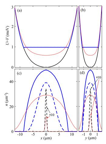
FIG. 2: (a,b) The IX energy profile in the bare diamond-shaped trap (black) and screened diamond-shaped trap for T = 50 mK (blue thick) and 10 K (red narrow). (c,d) The corresponding IX density distribution *n* (solid) and ground state density distributions  $n_0$  (dashed). For the screened trap in (a-d), the IX number in the trap N = 750, interaction parameter  $g = 20 \ \mu \text{eV} \cdot \mu \text{m}^2$ .
