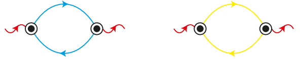
FIG. 3: Ultrasonic attenuation due to collective superconducting modes. Left figure shows contribution of the amplitude mode, when a phonon (red line) falls apart into two amplitude modes (blue lines). Exactly same process happens via phase modes (yellow lines), shown on the right.
