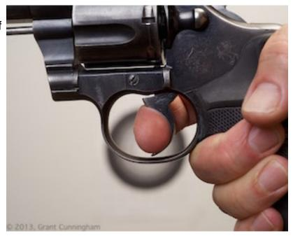
Revolvers that have had action jobs might be a well under those figures. Keep in mind that double action triggers under 9lbs need to be carefully tested, as low weights are usually the result of spring replacements or alterations — either of which can result in erratic ignition.
