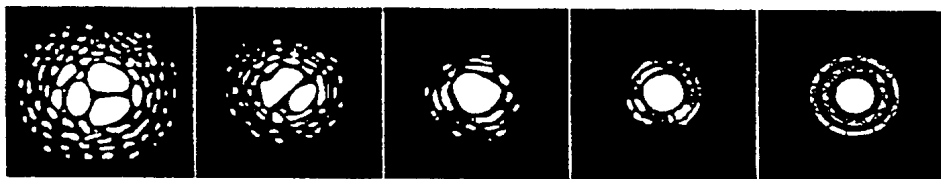
Figure 8-1 Seeing conditions directly affect image quality. These drawings represent a point source (i.e., star) under bad seeing conditions (left) to excellent condition (right). Most often, seeing conditions produce images that lie somewhere between these two extremes.
