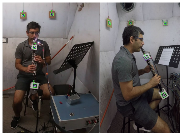
Figure 2. One of the authors demonstrating the use of the sensor-fitted clarinet, and the use of ArUco markers for clarinet position tracking (from [16]).
