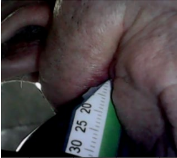
Figure 3. The mouthpiece fitted with a coloured scale used for tracking the lip position on the mouthpiece (from [16]).
