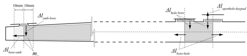
Fig. 2. The geometry and adjustable parameters of the modern flute impedance model. Bore segments and tone hole segments are modelled by cylindrical sections; head joint and embouchure hole modelled by conical sections. The adjustable parameters include five end corrections and one energy loss factor localized at the embouchure region.
