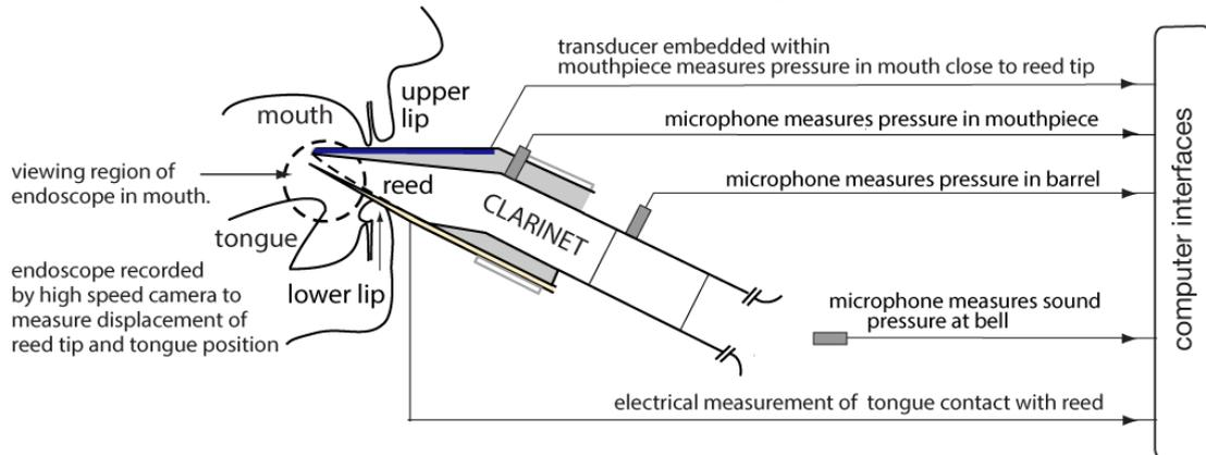
Figure 1 – A schematic of the experimental apparatus for measuring human players.
