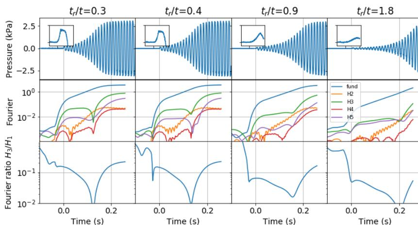
Figure 5 – Barrel pressure and its frequency components in transients on a playing machine.
