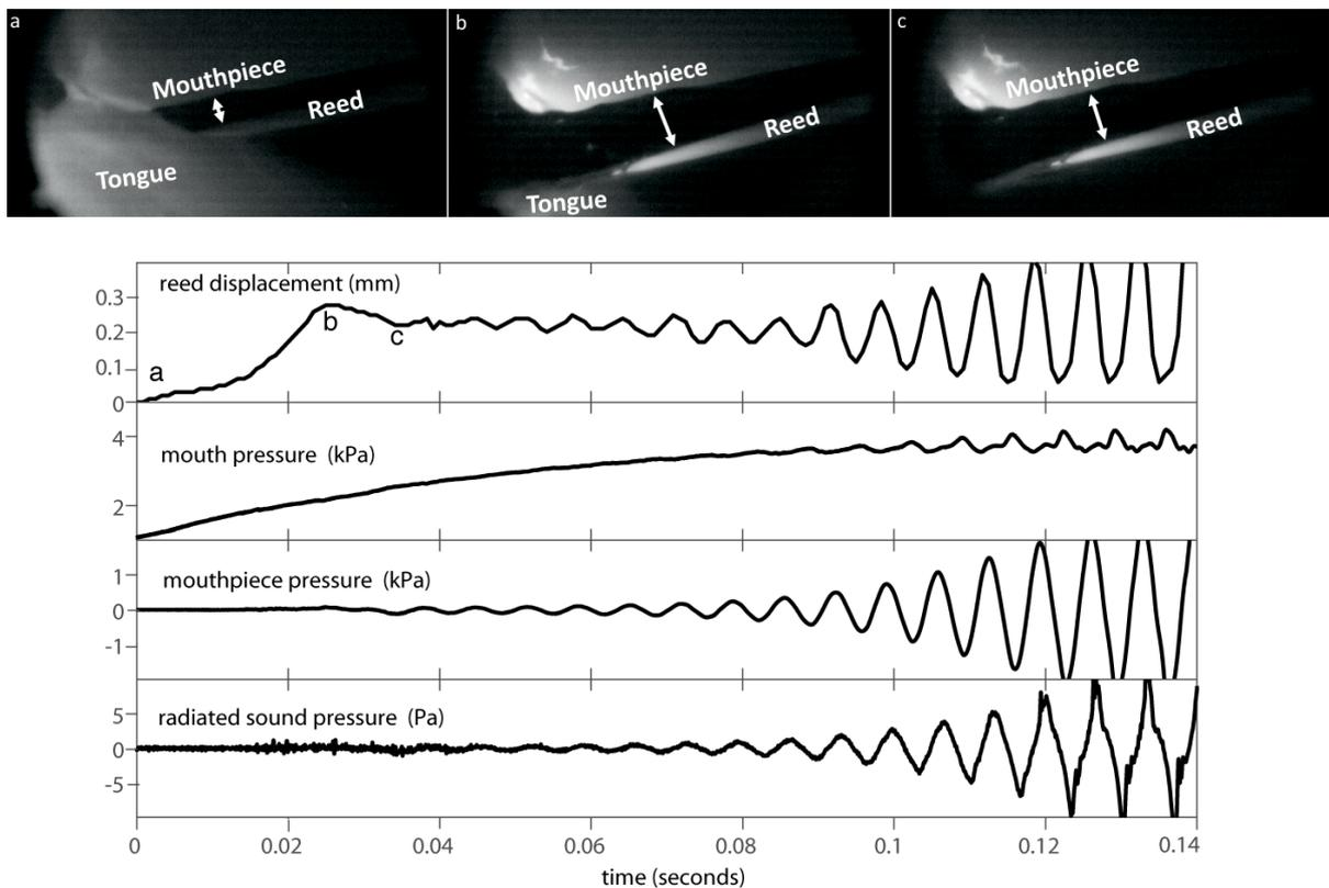
Figure 2 – The images (a, b, c) from the high-speed endoscope video show the labelled points on the graph of reed displacement from its initial position. The lower graphs show pressures in the mouth and mouthpiece and at the bell. An experienced player plays written E3, D3 concert (147 Hz), with normal tonguing. Details in Inwood *et al.* [12].
