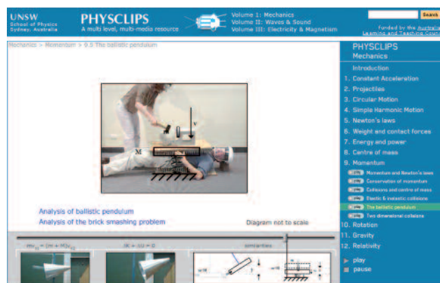
Fig. 2. This screen grab shows a section that discusses similarities in different problems. The ballistic pendulum (icons at lower left) involves an inelastic collision (momentum approximately conserved) and a pendulum swing (mechanical energy approximately conserved). In the circus stunt of the main picture, an inelastic collision of hammer and brick is followed by a (happily elastic) deformation of the presenter's chest.
