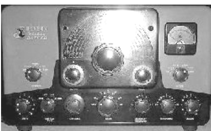
The E.F. Johnson Viking Ranger transmitter manufactured between 1954 and 1961. It operates between 160 and 10m, including the 11-meter band, with 75 W in CW and 65 W in AM. (Lombry, Page 11).
