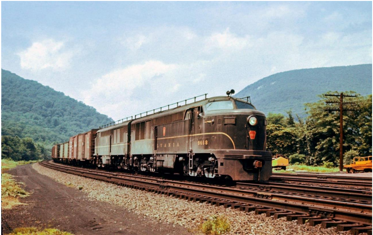
Pennsylvania Railroad locomotives, circa 1959, equipped with Trainphone. Note the handrail-like antennas on the roofs.
