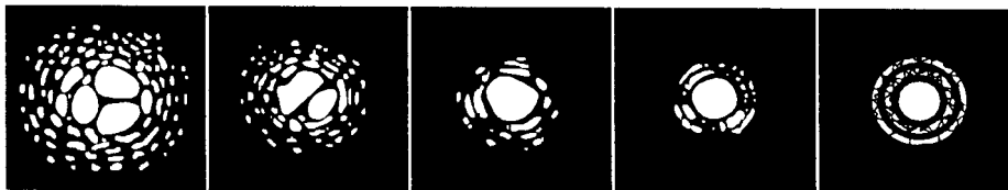
Seeing conditions directly affect image quality. These drawings represent a point source (i.e., star) under bad seeing conditions (left) to excellent conditions (right). Most often, seeing conditions produce images that lie some where between these two extremes.
