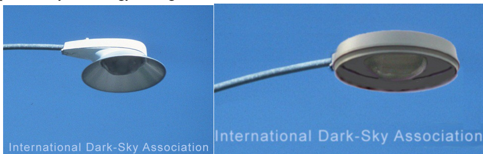
Figure 5. Extreme cases: fully shielded fixtures with prismatic glass (semi-cut-off). They fulfil the requirement of 0 cd/klm at 90 degrees and beyond.
