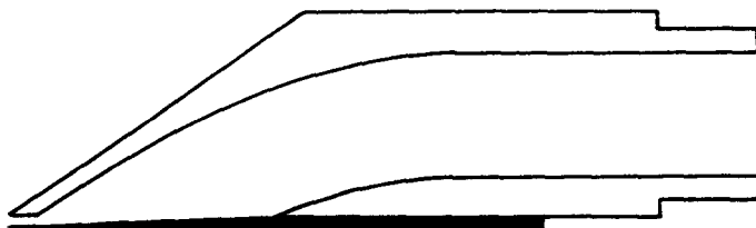
Fig. 2. The acoustic generator in a clarinet or saxophone consists of a flat cane reed, clamped against a slightly curved window in a rigid mouthpiece.
